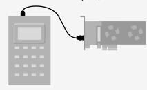
2. Luna PED Firmware 2.8.0 and newer is powered via the USB connection. If you are using Luna PED Firmware 2.7.1, connect it to power using the Luna PED DC power supply.
