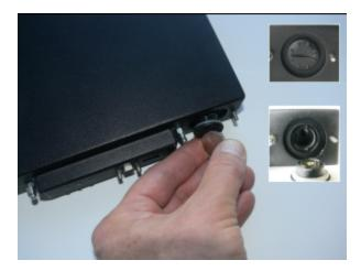
**3.** If you are replacing the old battery, remove it from the battery compartment.
